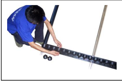
Remove all the covers of tube holder
